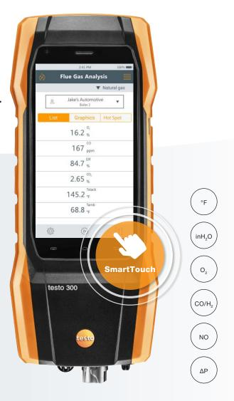
Truly smart combustion analysis: that is what the testo 300 stands for. The compact combustion analyzer is fully operated via the large touch display - you can see all the measuring values without scrolling. The scratch-resistant screen in embedded in a robust housing which remains reliable even in tough day-to-day working conditions. Menus for the most important measurements are already stored in the testo 300 and reliably guide you through the relevant application.
