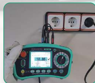
Loop test from a wall socket
