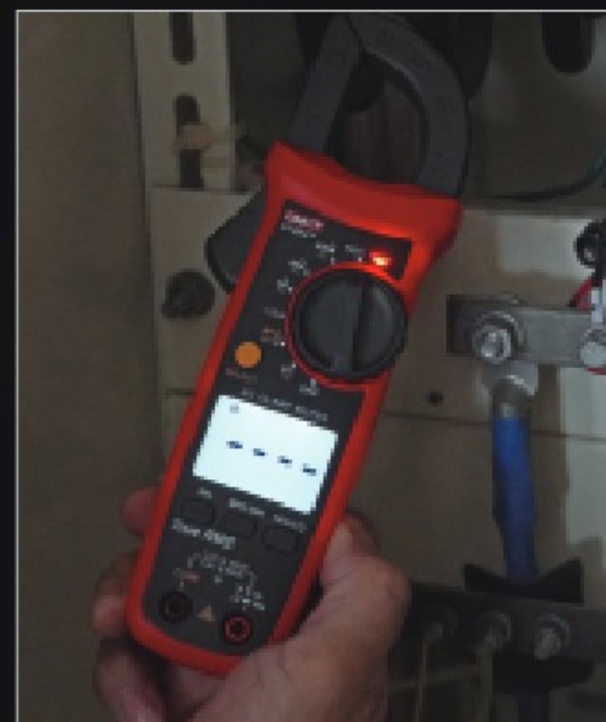
NCV multi-segment display and audio/visual alarm
