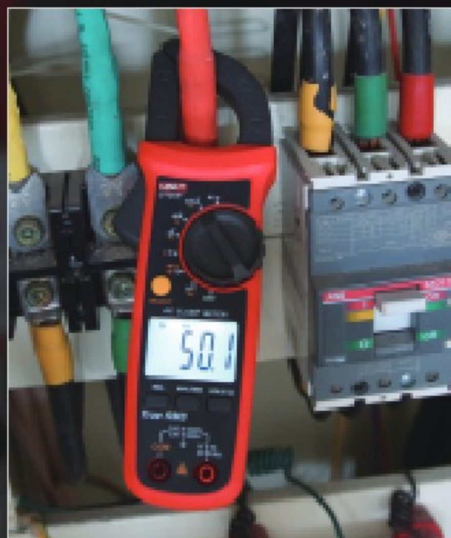
High voltage (600V) frequency measurement
